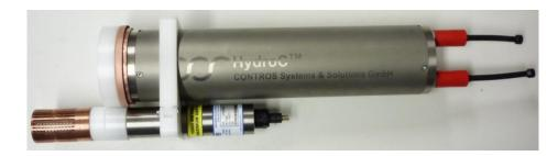
Fouling has no direct effect on the measurement as the membrane is not used as a sensing component within a HydroC, but solely as a phase boundary between water and internal headspace.
